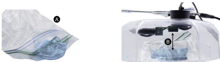
Figure 4. Cooling system placed beneath lid
