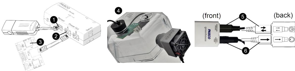
Figure 1. *//control.Node*, Greenhouse Sensor, and Fan Setup
