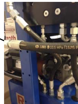
11 – Connection hose Overflow– 1/2"
