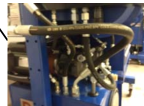
10 – Connection hose Sight glass drain – 3/4"
