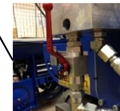
6.1 – Shut-off valve Drain valve
